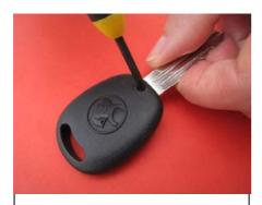
Unscrew holding screw located at the back of your remote key.
