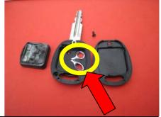
Separate back part of the cover from the key and pull your remote apart. If your buttons are already missing you may still have spring metal plate attached to the inside of remote.
